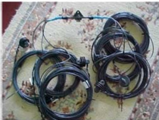
Figure 7: Direct Exchange Copper Piping
